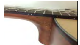
14th fret heel to body connection
